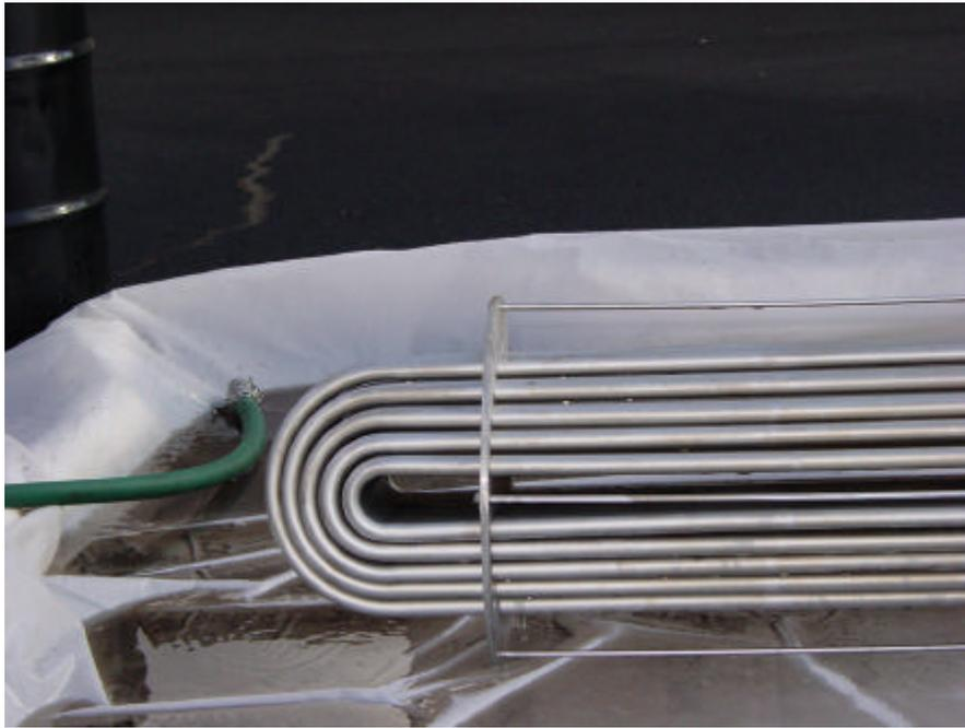
**Figure 10:** U2A reactor internal view after approximately 100 days operation. This reactor had processed 1,500,000 lb of urea containing about 4,500 lb of formaldehyde. This picture was taken immediately following removal of the tube bundle.
